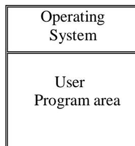
**Figure 1.2 Memory layouts for a simple batch system.**
