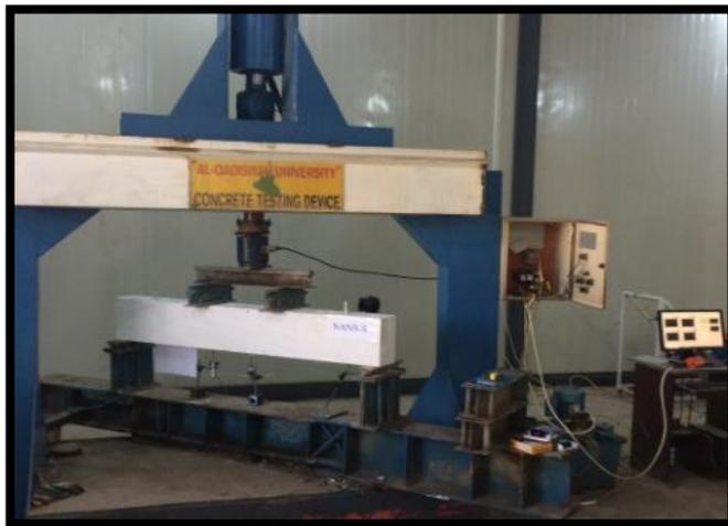
Figure 2. Testing machine and load pattern
