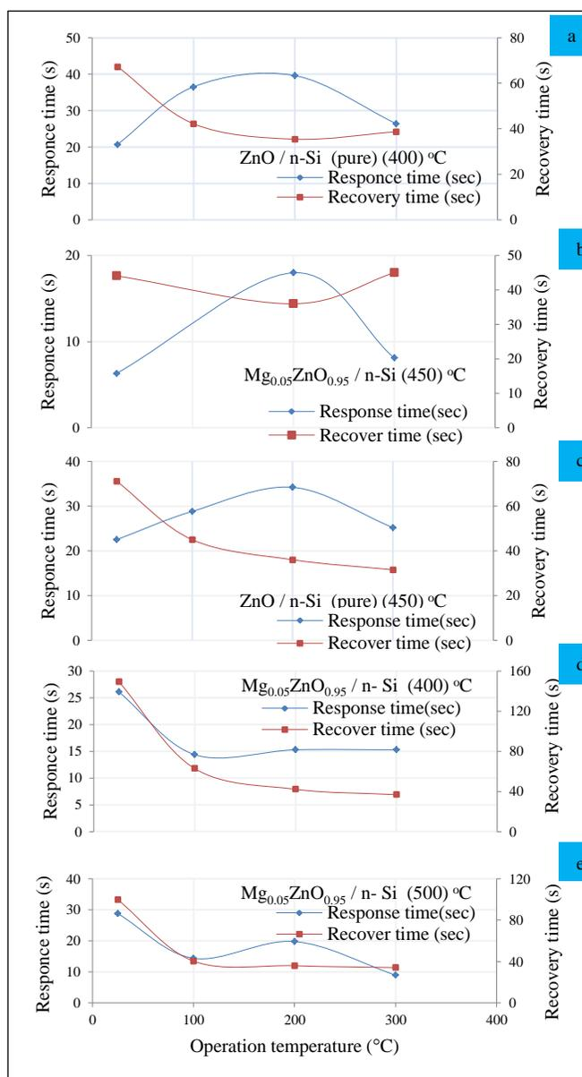
Fig.5: The variation of response time and recover time with different operating substrate temperatures for ZnO/n-Si and  $Mg_{0.05}ZnO_{0.95}/n-Si$  sensor at different temperatures (400,450, and 500) °C.
