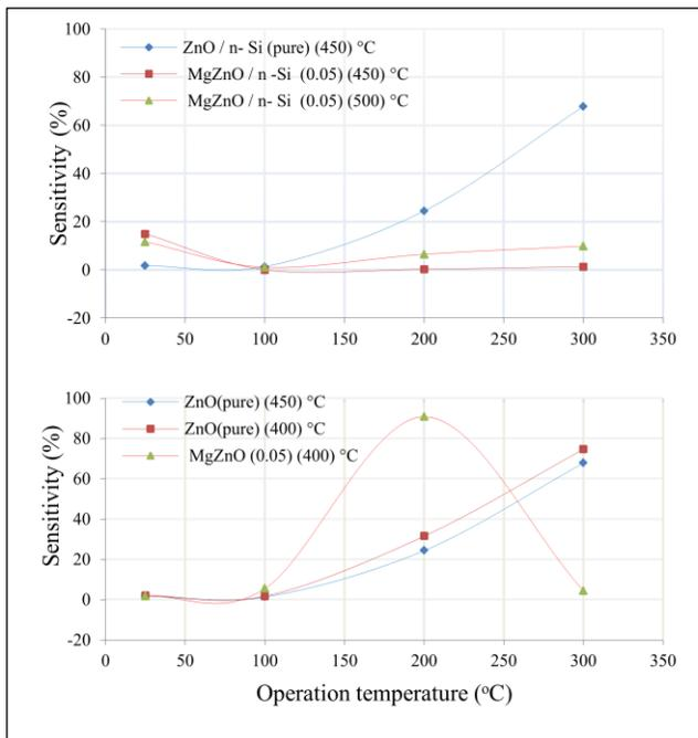
Fig.4: The variation of sensitivity with the different operating temperature of the ZnO/n-Si, and doped  $Mg_{0.05}ZnO_{0.95}/n-Si$  gas sensor at different temperatures (400,450,and 500) °C.
