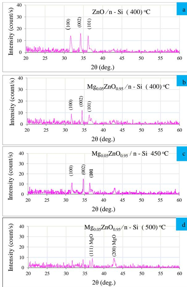
Fig.1: XRD patterns for ZnO/n-Si and doped  $Mg_{0.05}ZnO_{0.95}/n-Si$  gas sensor at different temperatures (400,450, and 500)  $^{\circ}C$ .
