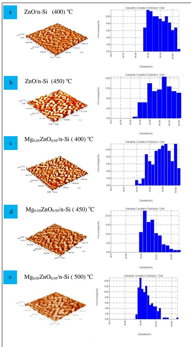
Fig.3: 3-D AFM image and granularity accumulation for ZnO/n-Si gas sensor and  $Mg_{0.05}ZnO_{0.95}/n-Si$  with different temperature (400,450, and 500) °C.
