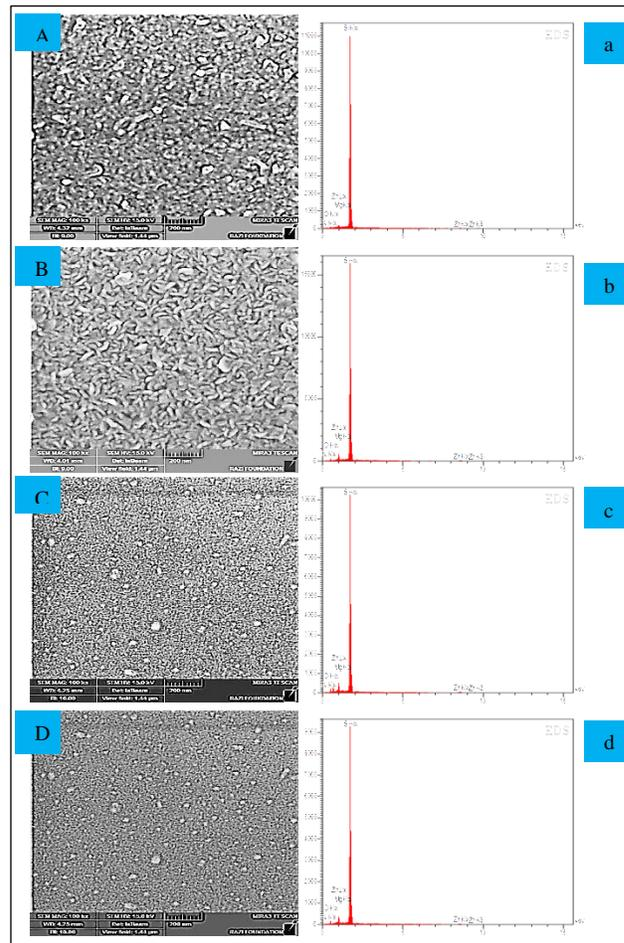
Fig.2: FESEM and EDS for ZnO/n-Si, and doped  $Mg_{0.05}ZnO_{0.95}/n-Si$  gas sensor at different temperatures(400,450,and 500)  $^{\circ}C$ .
